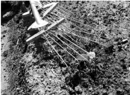
Vibrating weeding broom with four broom units in series.
